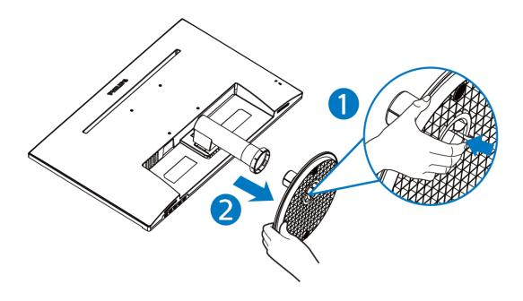
2. Press the release button to detach the base column.
