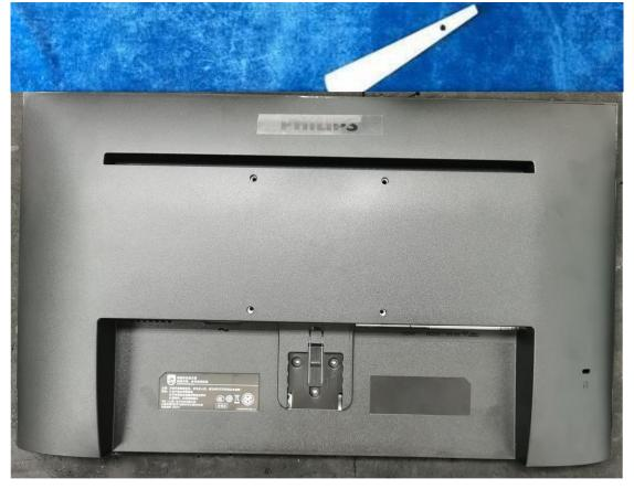
5. Remove the rear cover, then take off all of the tapes and disconnect the connectors.
