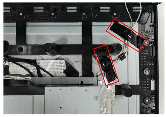
5. Remove the rear cover, then take off all of the tapes and disconnect the connectors.
