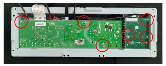
11. Remove screws to get middle frame and panel.
