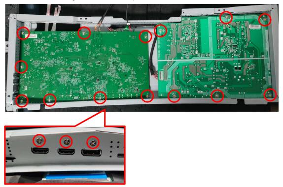
10. Remove screws to get middle frame and panel.
