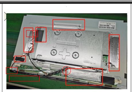
Separate the MAINFRAME and PANEL
