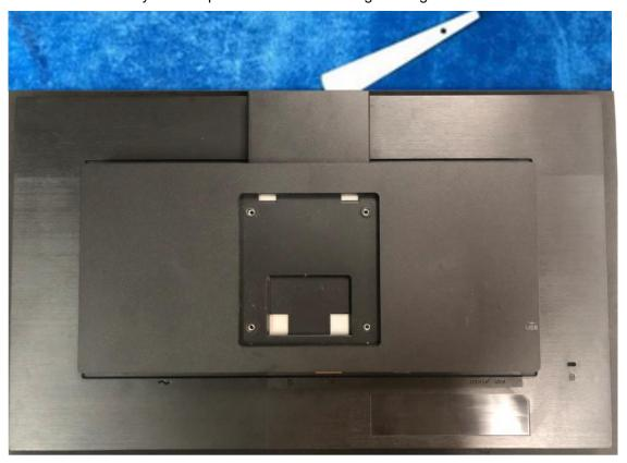
4. Remove the tapes and disconnect connectors.
