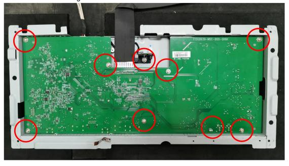
8. Remove screws to get middle frame and panel.
