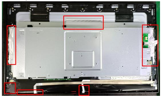
6. Remove tape and disconnect connectors.
