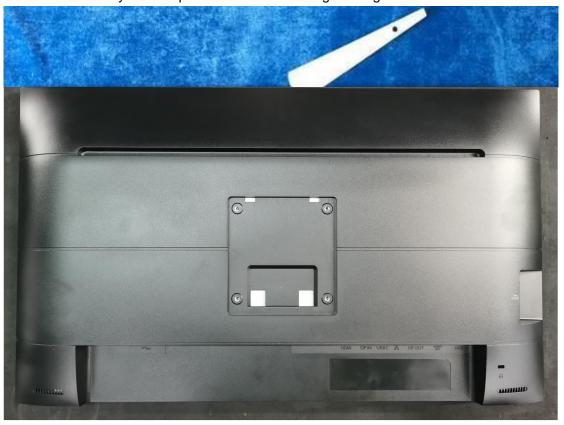
4. Throw the rear cover from one side, then take off the tape and disconnect the connector.
