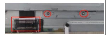
Disconnect all the cables, and tear out all the tapes to separate the main frame from panel.
