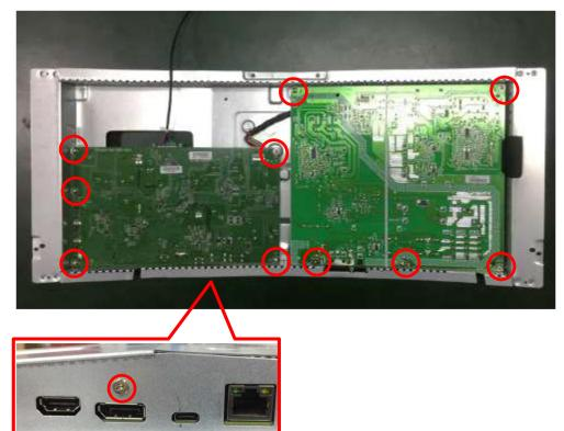
10. Remove screws to get middle frame and panel.
