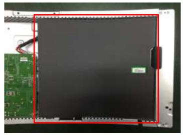
9. Remove screws to get main board and power board.
