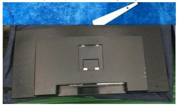
4. Take off the tape and connector then remove the rear cover.
