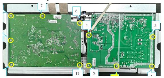
10. Remove screws to get middle frame and panel.
