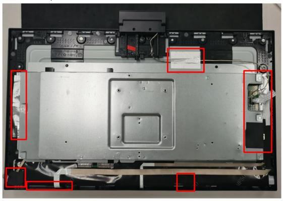
6. Remove tape and disconnect connectors.
