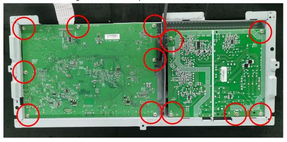
10. Remove screws to get middle frame and panel.
