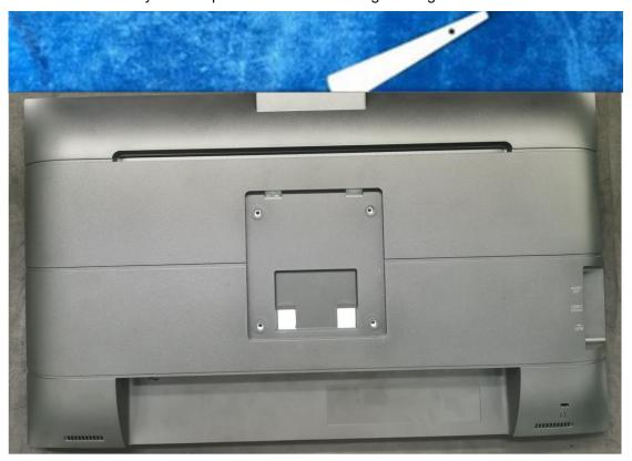
4. Take off the tapes and connector then remove the rear cover.
