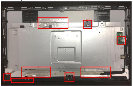
6. Remove tape and disconnect connectors.
