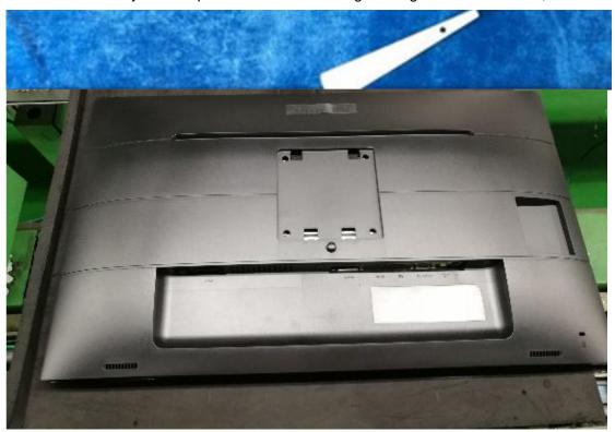
4. Throw the rear cover from one side, then take off the tape and disconnect the connector.
