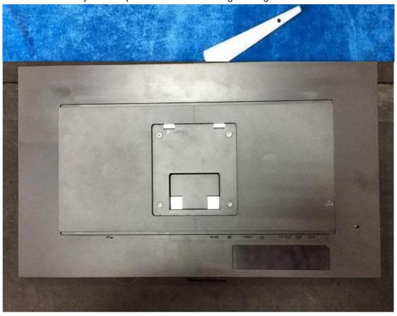
4. Remove the rear cover, then take off all of the tapes and disconnect the connectors.
