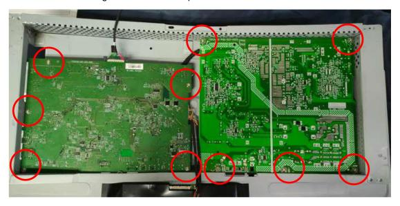
10. Remove screws to get middle frame and panel.
