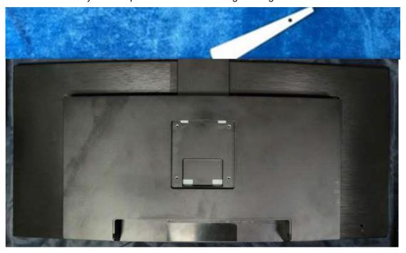
4. Take off the tapes and connector then remove the rear cover.
