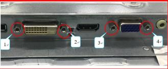
3. Remove the screws to remove the Main board. Power board
