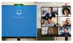
This Philips monitor comes with built-in 5MP webcam, noise cancelling microphone, and speakers. Making it perfect for working from home and collaborating remotely. Equipped with advanced sensors for Windows Hello™ facial recognition, which conveniently logs you into your Windows devices in less than 2 seconds. The physical camera switch offers extra privacy when not in use. The noise-cancelling microphone and dual 5-watt integrated speakers deliver clear communications.
