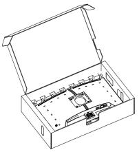
2. While keeping the release button pressed, tilt the base and slide it out.
