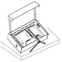
While keeping the release button pressed, tilt the stand and slide it out.
