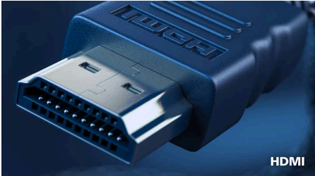
An HDMI-ready device has all the required hardware to accept High-Definition Multimedia Interface (HDMI) input. A HDMI cable enables high-quality digital video and audio all
