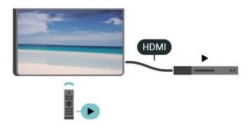
HDMI CEC (Consumer Electronic Control) must be switched on on the TV and the connected device.
