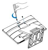
2. Move the stand into position as shown in picture. Then use a screwdriver to remove the screws, and then detach the stand from the monitor.
