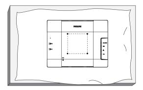
Ŷ M4 \* (10+X) mm (X=Thickness of Wall mount BKT) 100mm x 100mm
