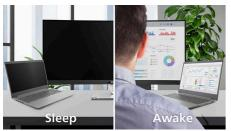
This monitor's PowerSensor 2 feature reduces energy consumption by detecting when users move closer and further away from the screen. After switching the OSD setting to "User", you then need to adjust the settings in Windows 11 for this feature to function properly. When these adjustments are made, the monitor and connected PC/laptop will wake when someone approaches it and sleep when someone walks away, effectively reducing the amount of wake
