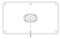
AC IN: Connect the AC cable to get power supply.
