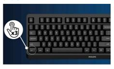
Unlike traditional built-in KVM monitor buttons, the smart KVM allows for switching between sources with the click of a button on your keyboard. When all devices are properly connected, users can easily switch between sources by clicking the "Ctrl" key three times.
