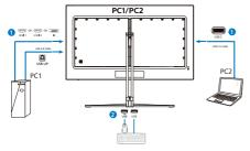
Enter to OSD menu. Go to KVM layer and select "Auto", "USB C" or "USB Up" to switch the control of peripherals from one device to another. Simply repeat this step for switching the control system using one set of peripheral.
