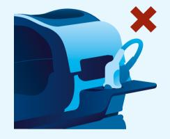
Store coil cables correctly after unplugging to avoid coil cables from hanging or being stretched.
