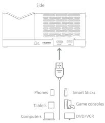
2 If the projector does not automatically switch to the correct input source, press → on the remote control to switch the input source to *HDMI*.
