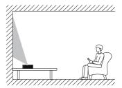
2 If the projection direction is incorrect, press on the remote control to access the projector's settings menu and select *Projector* > *Installation* > *Front Table.*
