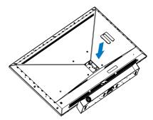
4. Due to the display rear design, make sure to secure 4 spacer nuts (provided in the box) before installing the wall mount bracket.over the hinge cover.
