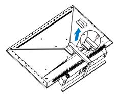
2. Loosen the assembly screws, then detach the stand from the display.
