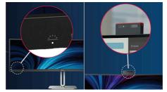
This feature allows for privacy and optimal collaboration when working in a busy office setting. To transmit to others that they are busy, users can simply press the Busylight hotkey located on the bottom left menu of the monitor bezel and the light located on the webcam will turn red. In addition to this, the Busylight feature can also sync with user's Microsoft Teams status.
