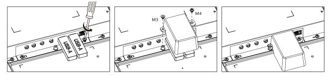
• Maximum suitable USB stick size: USB: 20(W)x10(H)x60(L) mm
