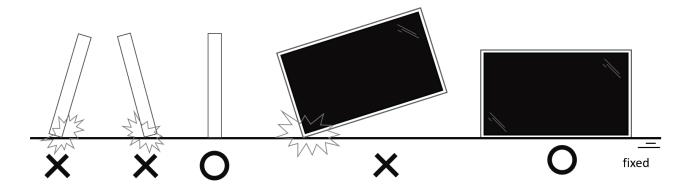
• Please keep vertically, no bending and torsion during moving the display.
