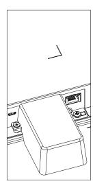
Maximum suitable size for the USB stick: USB: 20(W)x10(H)x60(L) mm
