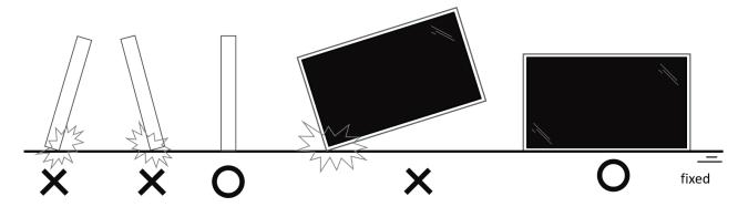
• Keep the display upright, without bending or twisting it while moving.
