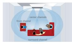
Ambisound technology produces truly embracing multi-channel surround sound from fewer speakers. It delivers an immersive 5.1 sound experience without the constraints of sitting position, room shape or size, and without the clutter of multiple speakers and cables. Through the combined effect of psychoacoustic phenomena, array processing and precisely angled driver positioning, Ambisound delivers more sound from fewer speakers.
