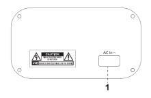
1 AC IN: Connect the AC cable to get power supply.
