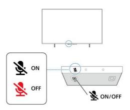
There is a switch button under the Far-Field Microphone, you can press to turn on or off the microphone. Normally the microphone is on ready status and the LED indicator light is off. If the microphone is turned off by pressing the switch button, the LED indicator light will be on to remind you the microphone is not ready.
