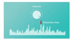
Anti-Clipping lets you play music louder and keeps it high quality, even when the battery is low. It accepts a range of input signals, from 300mV to 1000mV and keeps your speakers safe from damage by distortion. This built-in function monitors the musical signal as it goes through the amplifier and keeps peaks within the amplifier's range, preventing the audio distortion caused by clipping without affecting loudness. A portable speaker's ability to reproduce musical peaks decreases along with
