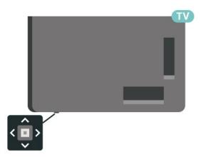
With the TV switched on, press the joystick key on the bottom of the TV to bring up the basic menu.
