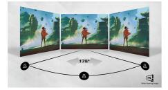
IPS displays use an advanced technology which gives you extra wide viewing angles of 178/178 degree, making it possible to view the display from almost any angle. Unlike standard TN panels, IPS displays gives you remarkably crisp images with vivid colors, making it ideal not only for Photos, movies and web browsing, but also for professional applications which demand color accuracy and consistent brightness at all times.
