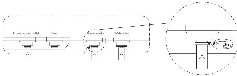
Note: The inlet water pressure should be within 0.3-0.7 MPa. If the pressure is too low, a pressure booster should be installed prior to the system. If the pressure is too high, a pressure relief valve should be installed prior to the system.
