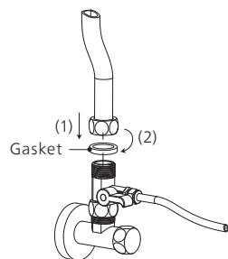
e. Switch off the three-way ball valve.
