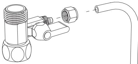
c. Install the three-way ball valve on the cold water valve.
