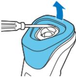
**2** Insert a flat-head screwdriver under the rim of the panel and pry off.
