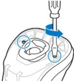
**3** Remove the two screws from the top with a torx or flat-head screwdriver.
