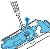
**6** Insert a flat head screwdriver on either side of the shaver body to release the hooks.
