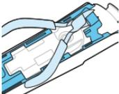
**5** Break the bridge on top with a wire cutter.
