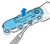
8 Bend the snap hooks aside and remove the transparent cover of the power unit.
