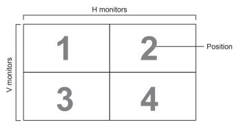
Example: 5 x 5 screen matrix (25 displays) H monitors = 5 displays V monitors = 5 displays
