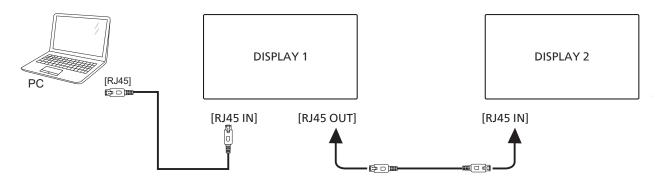
Connect laptop [USB] to adaptor and connect to [Control IN] of DISPLAY 1, connect the [Control OUT] connector of DISPLAY 1 to the [Control IN] connector of DISPLAY 2.
