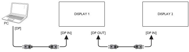
Connect laptop [DVI] to [DVI IN] of DISPLAY 1, connect the [DP OUT] connector of DISPLAY 1 to the [DP IN] connector of DISPLAY 2.
