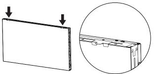
Install the top display carefully. After the displays are mounted, make sure you leave enough space between displays for removing the gap pad. If the pad is hard to release, adjust the position of the display to get enough space.
