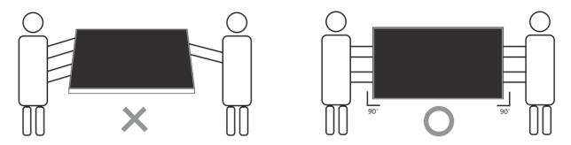
• Place the display vertically and its weight should spread evenly on the surface.
