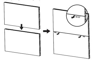
4. Apply another gap pad on the side surface and repeat the same process as step 3.
