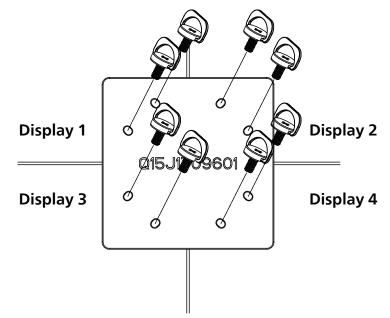
• Use the "Edge Alignment Kit-2" for two adjacent displays.
