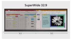
32:9 SuperWide 49" screen with 5120 x 1440 resolution is designed to replace multiscreen setups for a massive wide view. It's like having two 27" 16:9 Quad HD displays side by side. SuperWide monitors offer the screen area of dual monitors without the complicated setup.
