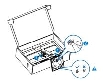
Note Secure the arrow of the base towards the front and fix to the column tightly.
