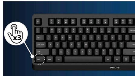
Unlike traditional built-in KVM monitor buttons, the smart KVM allows for switching between sources with the click of a button on your keyboard. When all devices are properly connected, users can easily switch between sources by clicking the "Ctrl" key three times.
