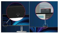
This feature allows for privacy and optimal collaboration when working in a busy office setting. To transmit to others that they are busy, users can simply press the Busylight hotkey located on the bottom left menu of the monitor bezel, and the light located on the webcam will turn red. In addition to this, the Busylight feature can also sync with users' Microsoft Teams status.
