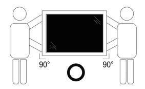
• Place the display vertically and its weight should spread evenly on the surface.
