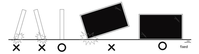
• Keep the display in a vertical position when moving it, no bending is allowed.
