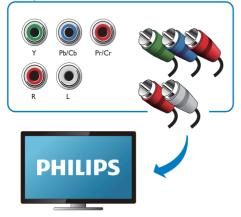
Connect a progressive scan TV through component video cables for higher quality video.
