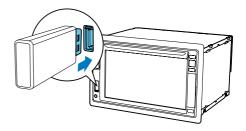
• To remove the USB storage device, switch the system to another source first.
