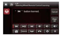
5 Repeat steps 3 and 4 to assign more functions to buttons on the steering wheel.
