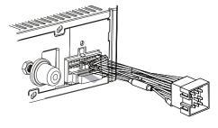
3 Connect the antenna and amplifier as illustrated, if applicable. You can connect the car audio to the amplifier through RCA-TO-RCA cables (not supplied).
