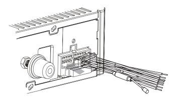
2 Connect the other end of the supplied standard connector to the unit.
