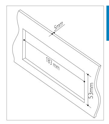
5 Install the sleeve into the dashboard and bend the tabs outward to fix the sleeve.
