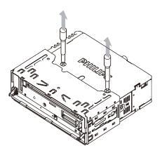
3 Remove the mounting sleeve with the supplied disassembly tools.
