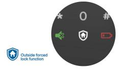
Before leaving home, you can touch the outside forced lock key to enable the function. In this mode, opening the door from inside the room will trigger an alarm. This feature can effectively warn you of security risks and upgrade the level of home security.
